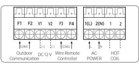
★ The output of hot coil terminal is AC 220 V / 230 V (The same as Indoor Unit's input Power)
